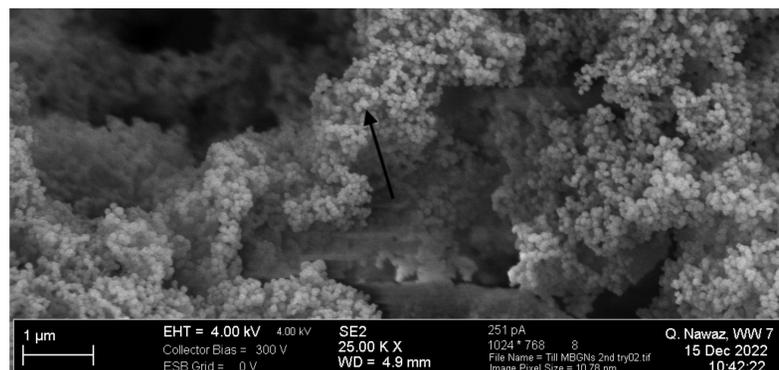
Figure 1: SEM image of mesoporous bioactive glass nanoparticles (MBGNs) which are intended for the reinforcement phase to a bioactive composite bone scaffold.
