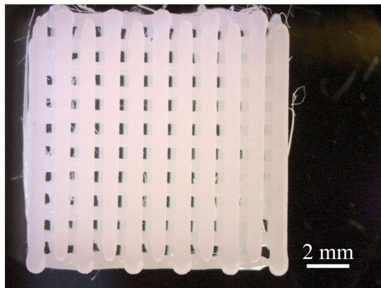
Figure 3: Light microscope camera image (Zeiss Axiocam 105 Color) of a PCL/MBGN (5 wt%) scaffold. Top view.
