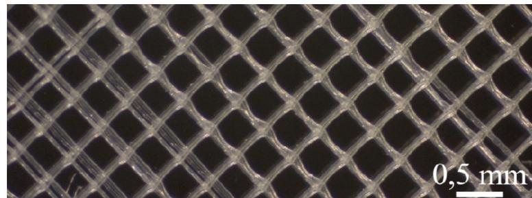
Figure 2: Light-Microscopy camera (Zeiss Axiocam 105 Color, Carl Zeiss AG) image of a scaffold produced using Melt-Electrowriting (MEW).
